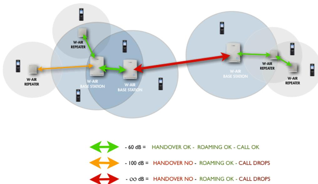
**Note:** For a good conversation and a correct handover between bases and Repeaters the dBm value must be between -75 and 0. Base stations cannot be connected with the help of repeater.
