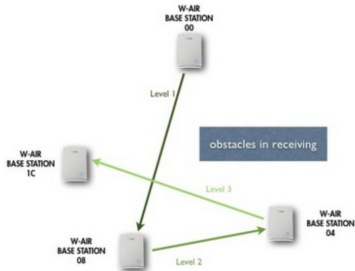
The value shown in the “DECT sync source” field indicates the real dBm value. Based on this value you can choose the best connection solution for your system, taking into consideration any obstacles present in the environment.
