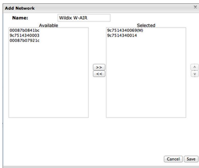
*Note: The first device becomes the Master of the network (M). The gateways make Radio sync with each other automatically to extend the work range if possible.*
